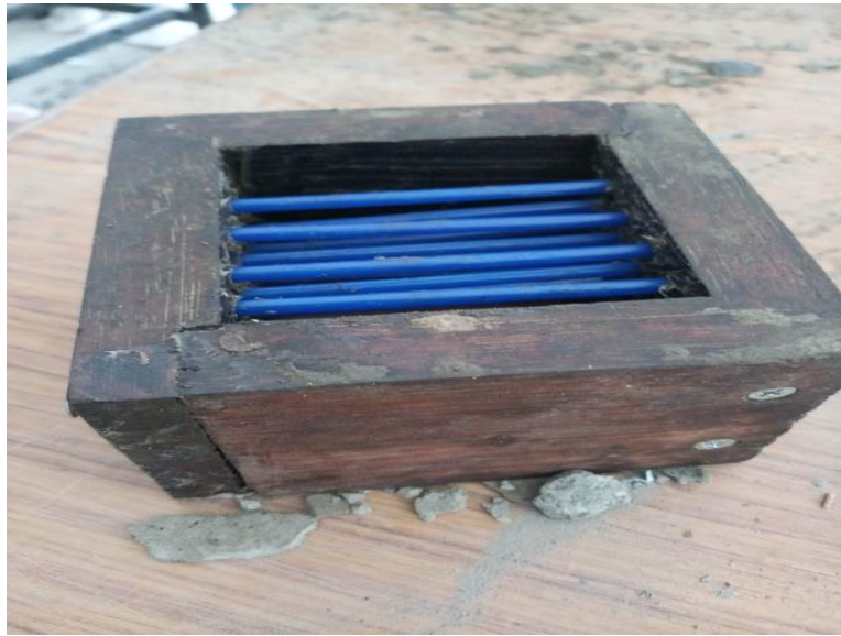
Fig 3.2:Placing of Pen Refills Onto The Wooden Mould
