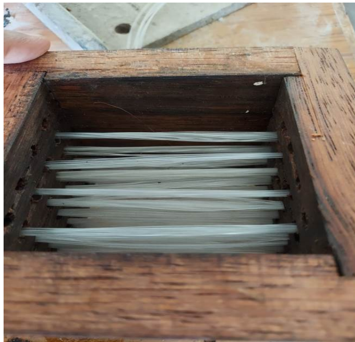
FIG 3.1: Placing of Optic Fibres Onto The Wooden Mould
