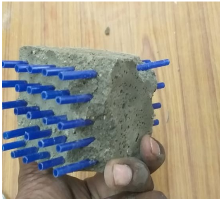
Fig4.1:Translucent Concrete Blocks Incorporated with Optic Fibres
